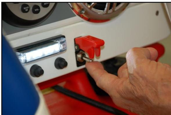
Your engine is equipped with an electric tilt safety switch. In order to lift the engine with electric tilt it is necessary to toggle the safety switch located below the stereo (as shown) at the same time you press the tilt up button on the handle of the control box. The engine should be in the straight ahead position before tilting the engine up. The tilt down button on the control box does not require pressing the safety switch at the same time.
