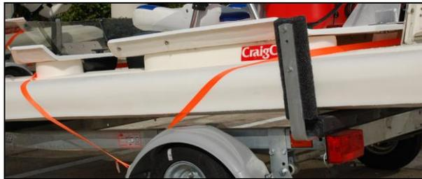
It is best to tighten the rear strap first. Notice the rear strap goes under the transom, not to the outside of the engine mount.
