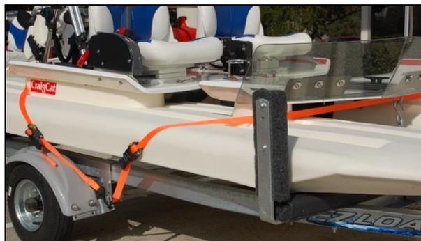
The front strap should be tightened last. Notice the front strap goes behind the safety chain.
